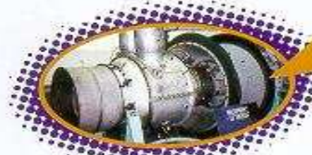
Figure 12: 2.5 MWe Gas turbine modified by Orenda, Canada
